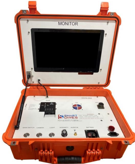
1 DIVER 1 CCTV MONITOR SYSTEM
